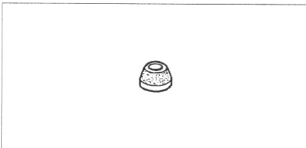
Head Pipe Outer Race Driver : 57001-1446
